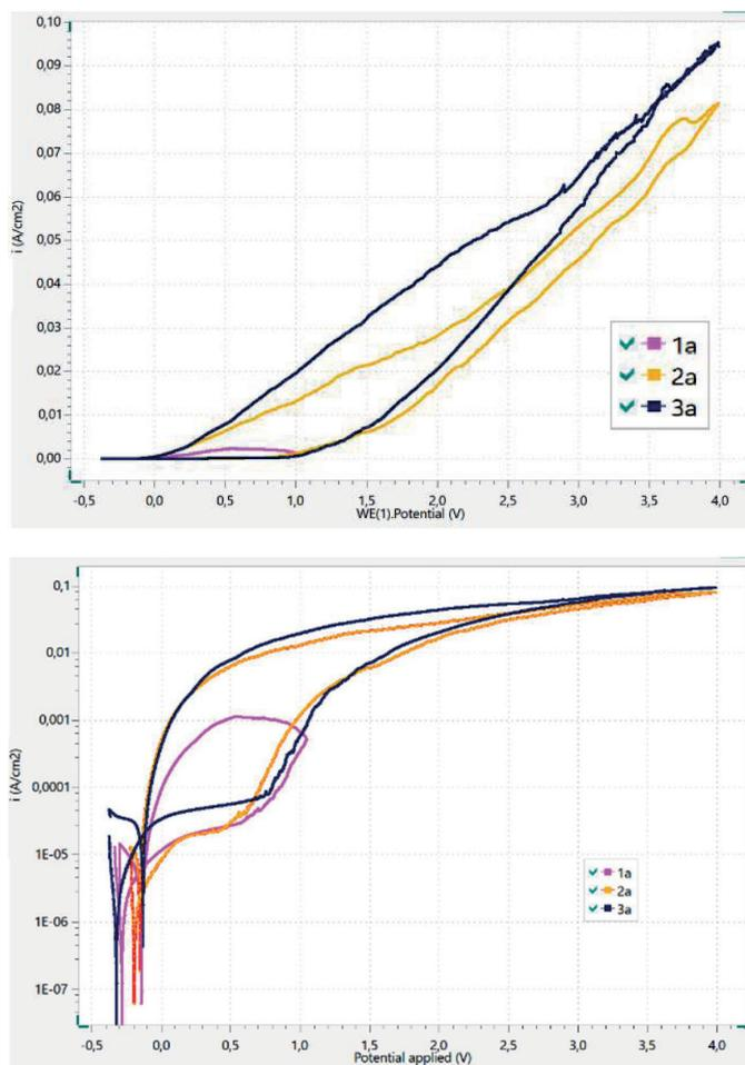
**Fig. 6.** Anodic polarisation curves for 316LVM steel without TiN layer
