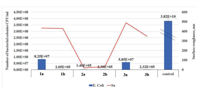
**Fig. 8. Results of bacterial adhesion in surface roughness values: 1 – sandblasted, 2 – polished, 3 – electropolished**
