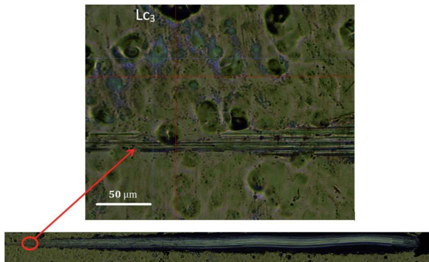
**Fig. 3. Result of the scratch test for 3b, electropolished with TiN layer**
