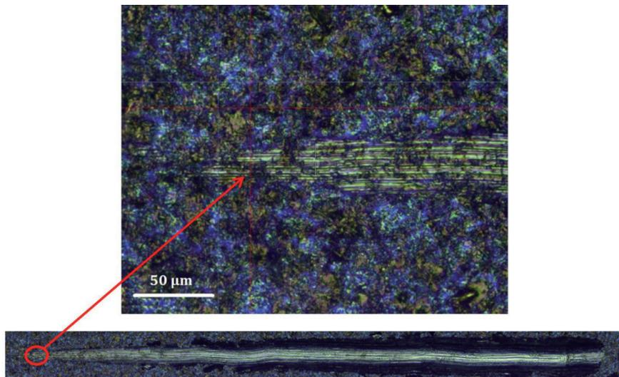
**Fig. 1. Result of the scratch test for 1b, sandblasted with TiN layer**
