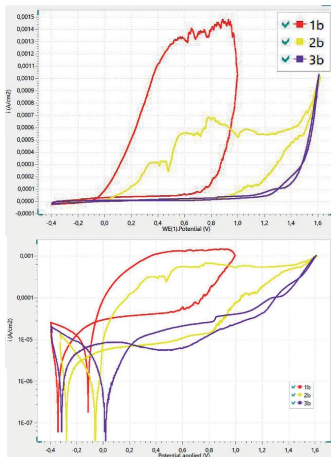
**Fig. 7. Anodic polarisation curves for 316LVM steel with TiN layer**
