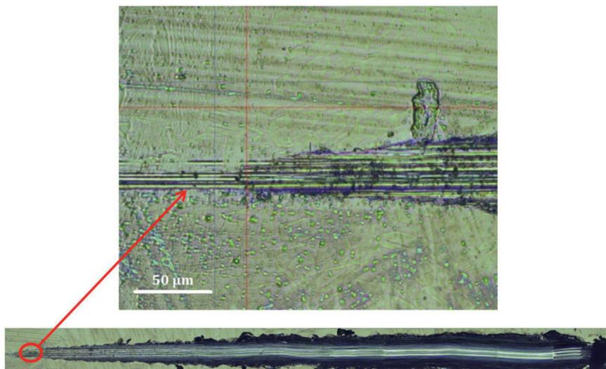
**Fig. 2. Result of the scratch test for 2b, polished with TiN layer**
