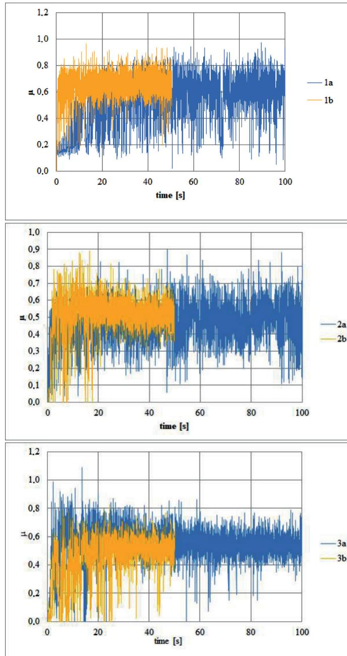
**Fig. 4. Results of tribological tests – without and with TiN layer**
