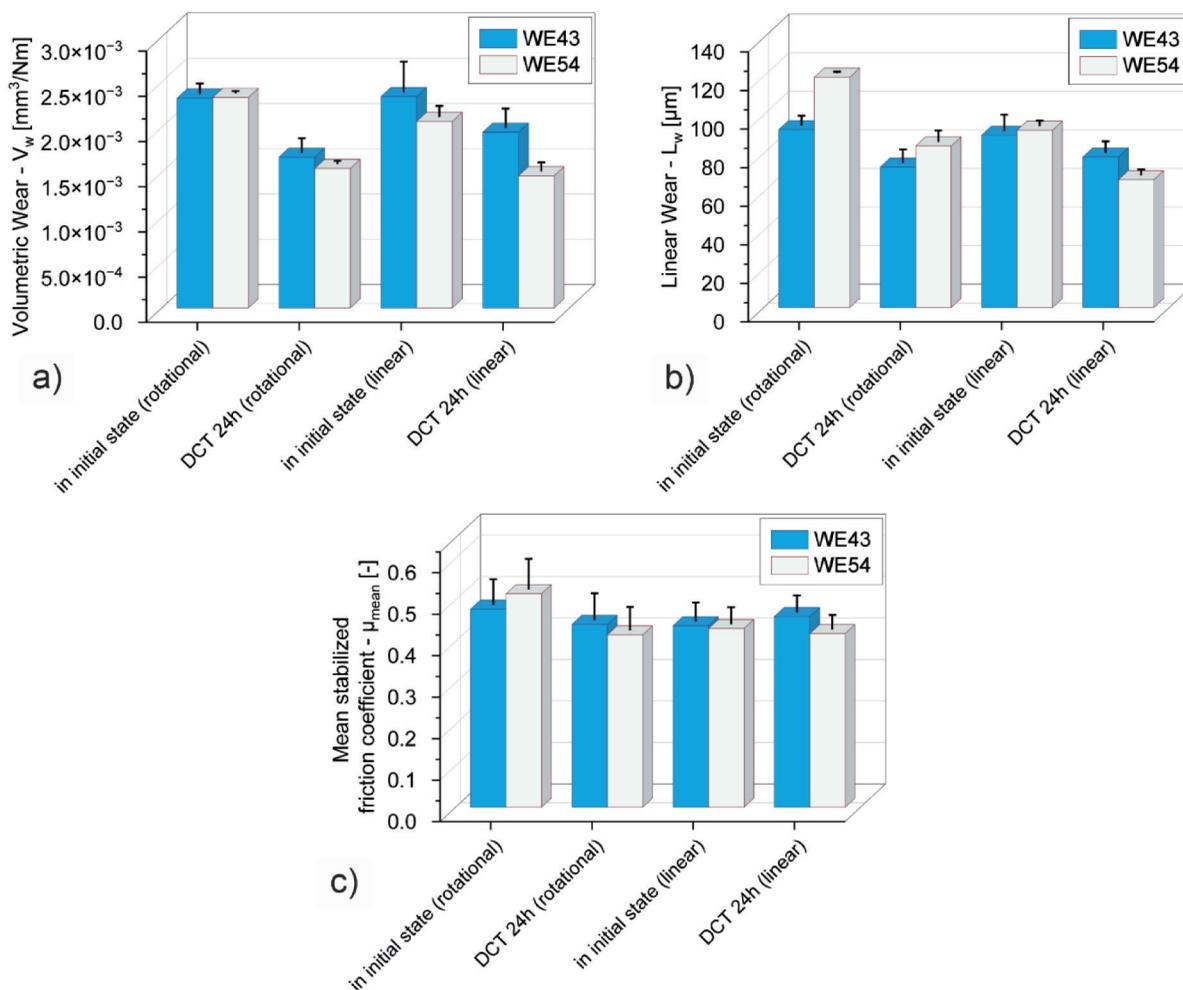
**Fig. 4. Changes in volumetric wear  $V_w$  – a), linear wear  $L_w$  – b) and stabilised friction coefficient  $\mu_{\text{mean}}$  of Mg alloys WE43 and WE54 in their initial state and after deep cryogenic treatment for 24 h**
