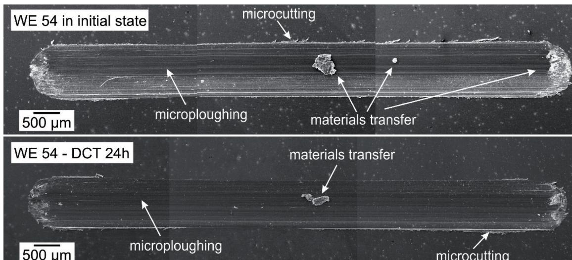
**Fig. 5. Morphologies of the wear traces of Mg alloy WE54 formed in reciprocating linear motion in the as-delivered state and after deep cryogenic treatment for 24 h**
