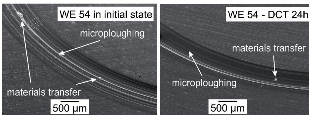
**Fig. 6. Morphologies of the wear traces of Mg alloy WE54 formed in rotary motion in the as-delivered state and after deep cryogenic treatment for 24 h**
