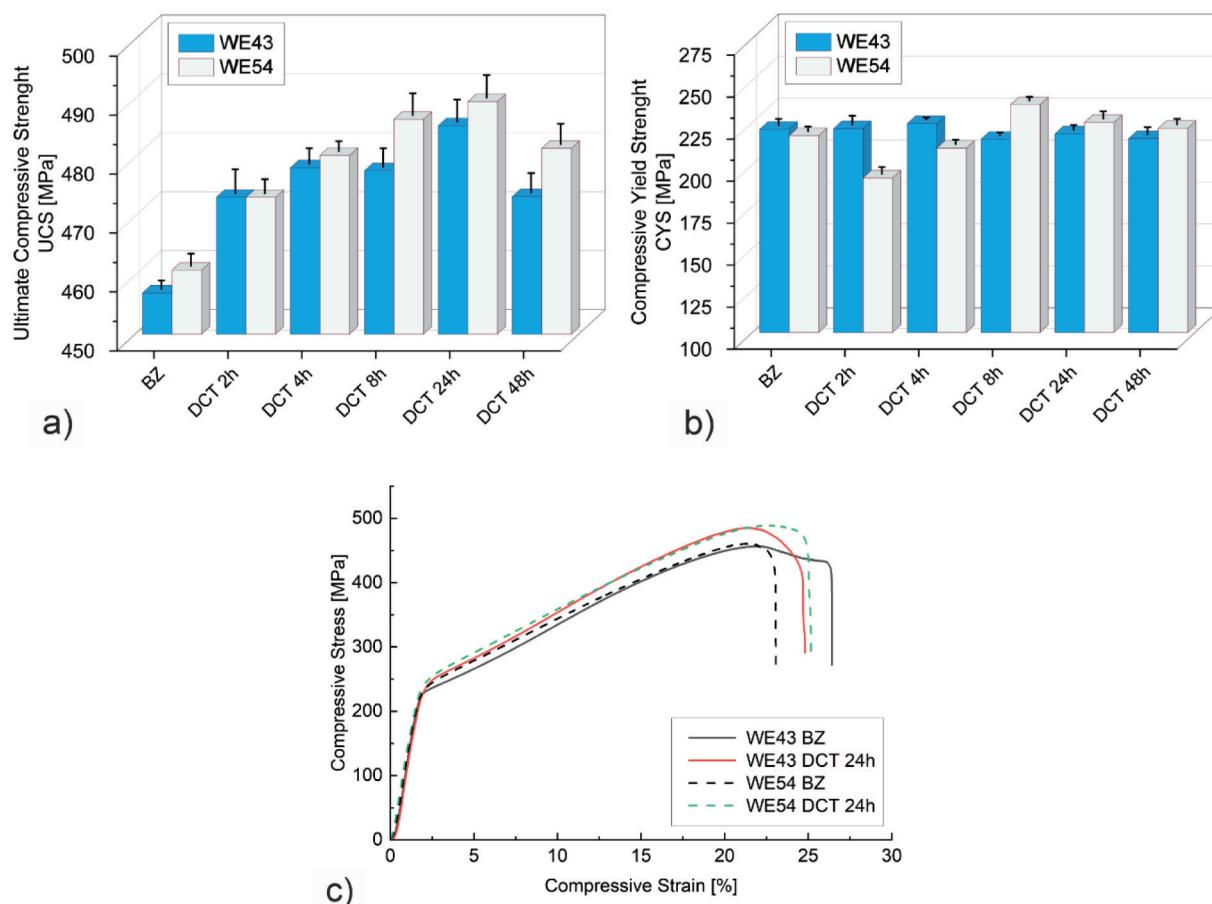
**Fig. 3. Compression test parameters of Mg alloys WE43 and WE54 after deep cryogenic treatment: compressive strength UCS ( $R_c$ ) – a), proof stress UYS ( $R_{c0.2}$ ) – b) and examples of compression curves for the alloys in their initial state and after sub-zero treatment for 24 h – c)**
