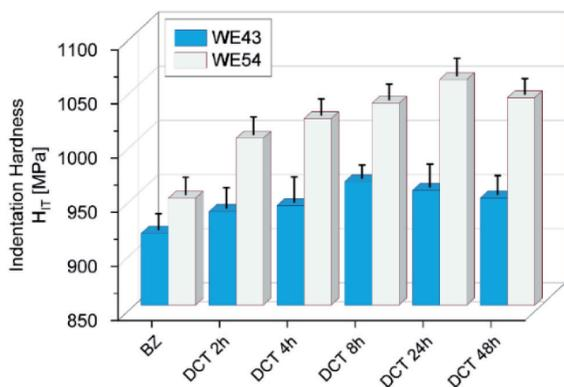
Fig. 1. Changes in hardness  $H_{IT}$  of alloys WE43 and WE54 with increasing time of deep cryogenic treatment
