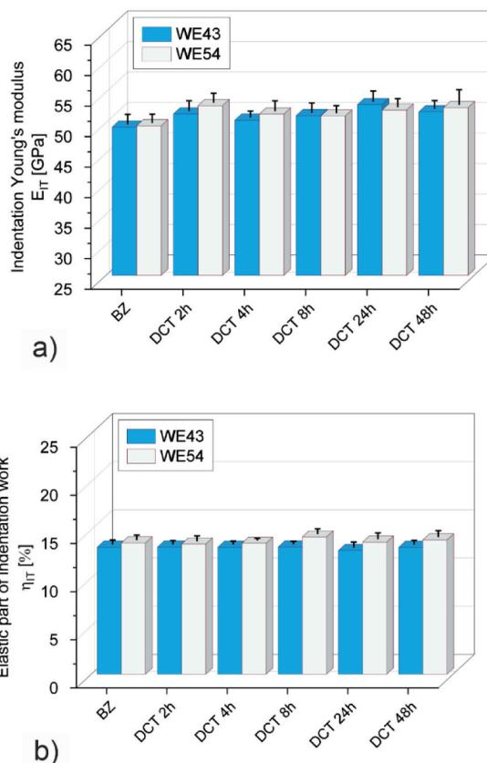
Fig. 2. Changes in Young's modulus  $E_{IT}$  – a) and in the percentage of the elastic component of indentation work  $\eta_{IT}$  – b) of alloys WE43 and WE54 with increasing time of deep cryogenic treatment
