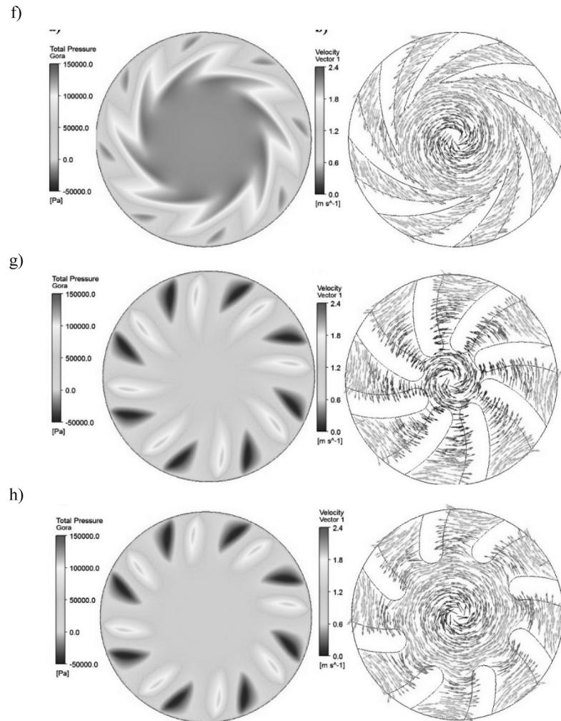
**Fig. 6. Contour diagrams of the spatial distribution of total pressure and the fluid velocity vector in the analysed bearings**
