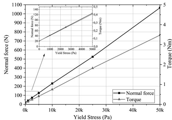
**Fig. 7. The relationship between the axial force and the friction torque as a function of the modelled fluid yield stress**
