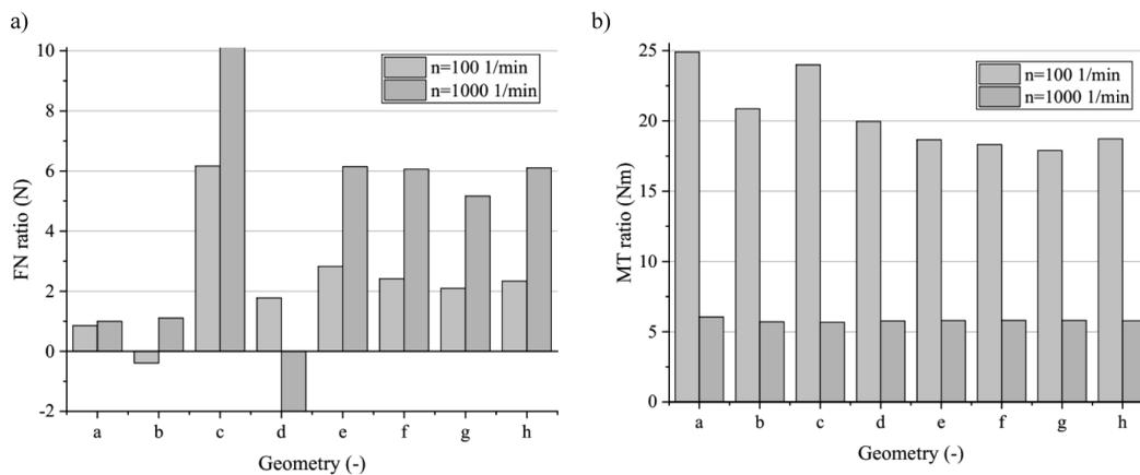
**Fig. 5. Plots of the relative change; a) axial force; b) friction moment**
