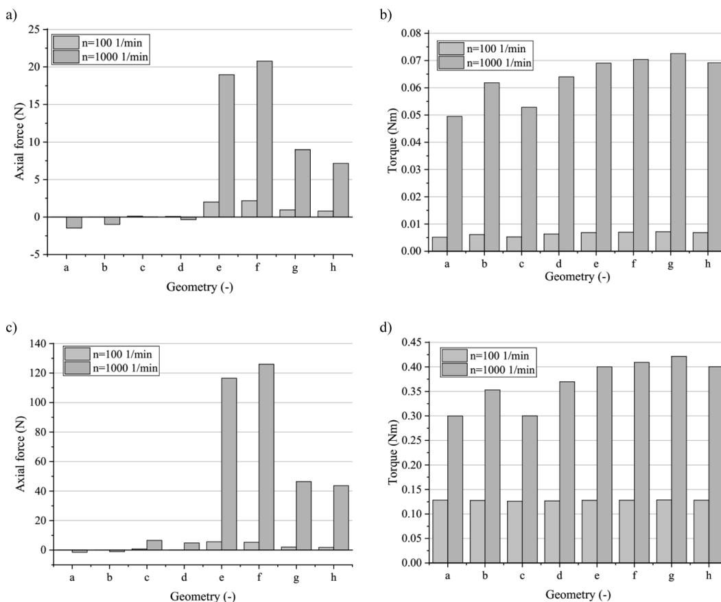
**Fig. 4. Results of simulation studies of axial force and friction torque for the tested geometries: a, b) fluid No. 1, c, d) fluid No. 5**
