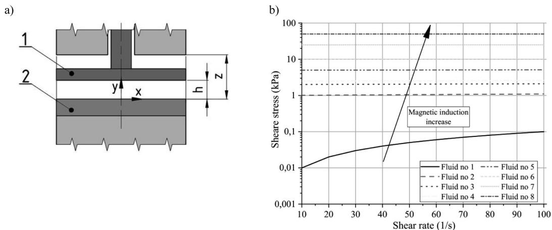
**Fig. 1. Scheme of the tested thrust bearing (a), flow curves of the modeled magnetic fluid (b)**
