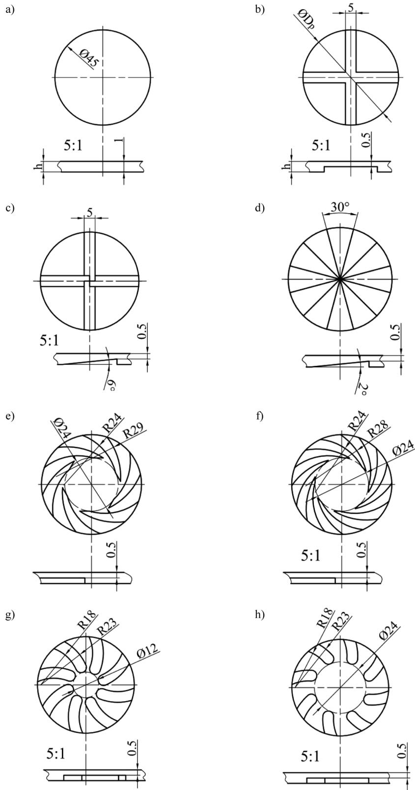
**Fig. 2. Design and dimensions of thrust bearing pads adopted for the simulation studies**
