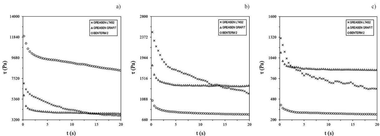
**Fig. 7. Dependence of shear stress on grease shear time for an average shear velocity of 50 mm/s. Lubricant temperature: a)  $-10^\circ\text{C}$ , b)  $20^\circ\text{C}$ , c)  $50^\circ\text{C}$**
