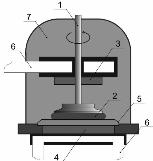
**Fig. 3. Diagram of the measuring head of the rotational rheometer used for testing: 1 – measuring spindle (with an upper sanded plate with a diameter of 40 mm), 2 – lubricant, 3, 4 – Peltier module (P-PTD200), 5 – bottom plate, 6 – cooling system, 7 – insulating and thermostatic collar (H-PTD200)**
