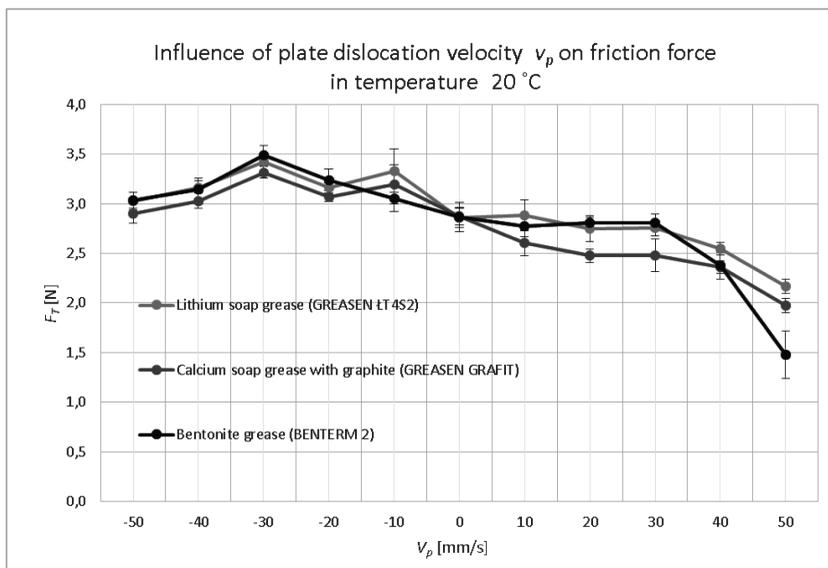
**Fig. 5. Influence of plate dislocation velocity on the value of friction force during rolling with sliding movement at 20°C**
