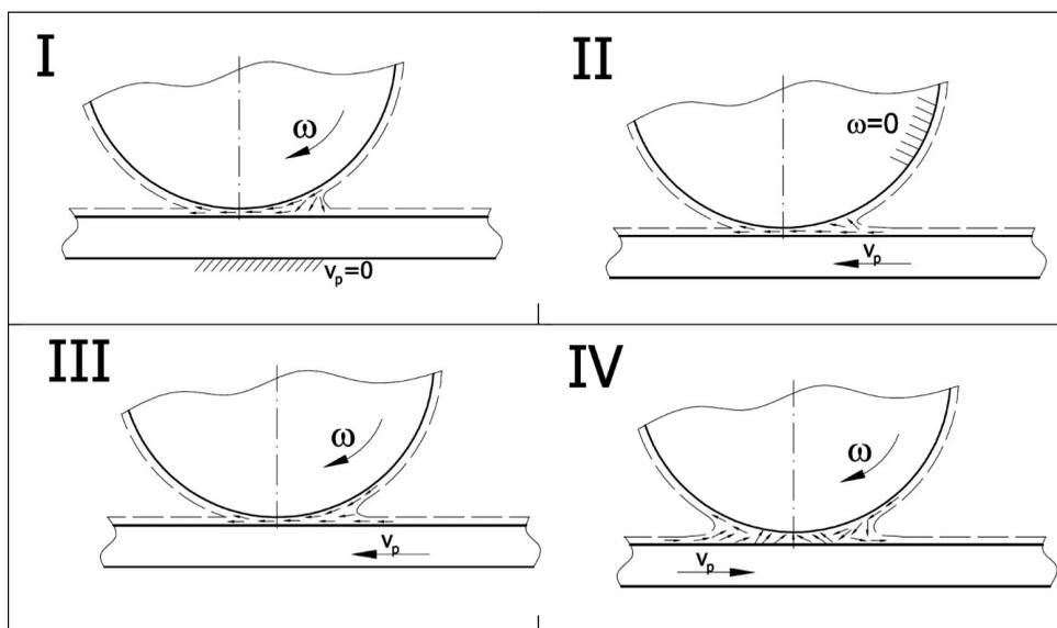
**Fig. 8.** The mechanism of lubricant flow in the friction joint (pair) for various kinematic cases: I – rotation of the roller with the stationary plate ( $v_p = 0$ ), II – motion of the plate with the stationary roller ( $\omega = 0$ ), III – simultaneous motion of the plate and rotation of the roller in this same direction (concurrent motion), IV – simultaneous dislocation of the plate and rotation of the roller but in opposite directions (opposite motion). Own study
