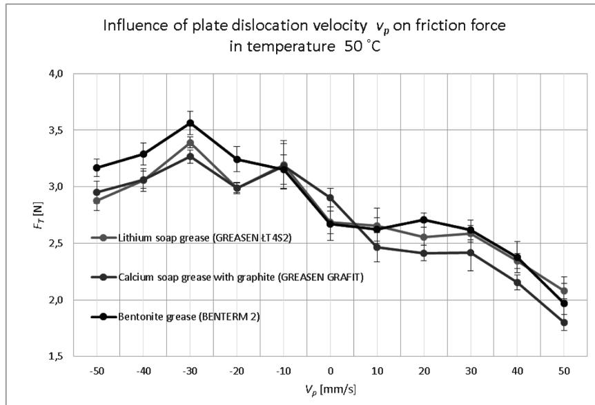
**Fig. 6. Influence of plate dislocation velocity on the value of friction force during rolling with sliding movement at 50°C**
