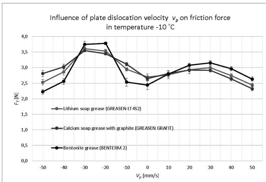
**Fig. 4. Influence of plate dislocation velocity on the value of friction force during rolling with sliding movement at -10°C**
