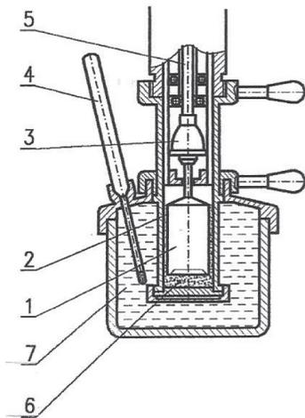
Fig. 4. Measuring head of the Rheotest 2.1 rheometer: 1 – internal measuring cylinder, 2 – external measuring cylinder, 3 – coupling, 4 – thermometer, 5 – drive shaft, 6 – lubricant tested, 7 – thermostatic agent
