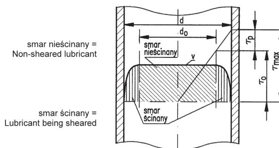
**Fig. 3. Distribution of shear stresses and velocities in grease flowing through a pipeline [L. 8]**
