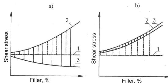
**Fig. 1. The main physicochemical (a) and geometric (b) impact on the shear stress value in the plastic grease composition with the filler: 1 – the course of shear stress in the grease without a filler, 2 – the influence of the geometrical factor on the shear stress value in the lubricant composition, 3 – the total effect of the geometric and physicochemical factor on the value of this stress [L. 4, 6]**
