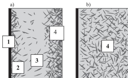
**Fig. 2. Formation of the surface and boundary layers in the grease flowing near the wall made of material, which (a) has the ability to adsorb the thickener particles, (b) does not have the ability to adsorb the thickener particles: 1 – material wall, 2 – surface layer (adsorbed particles of the grease thickener on the surface of the material wall), 3 – boundary layer (the area depleted of the thickener, with smaller structural viscosity), 4 – grease mass [L. 12]**
