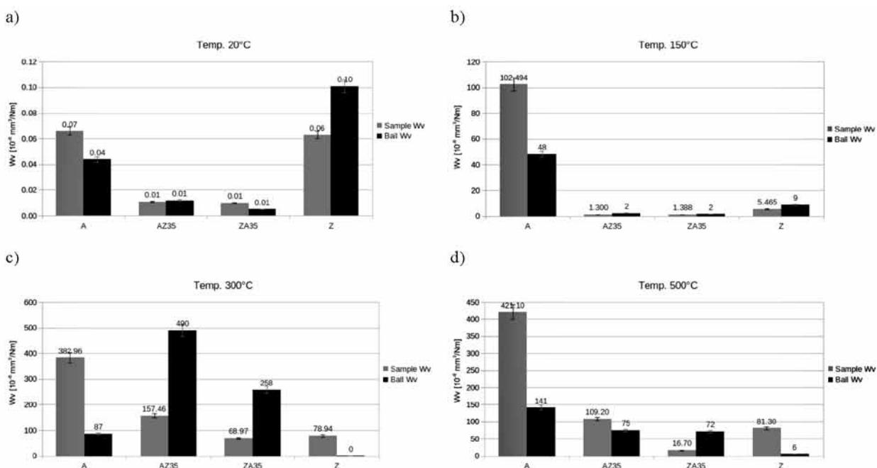
**Fig. 3. Wear rate of the sample and countersample tested at temperatures: a) 20°C, b) 150°C, c) 300°C, d) 500°C**
