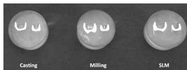
Fig. 5. Samples for micromechanical tests – axial cross-sections of crowns embedded in resin
