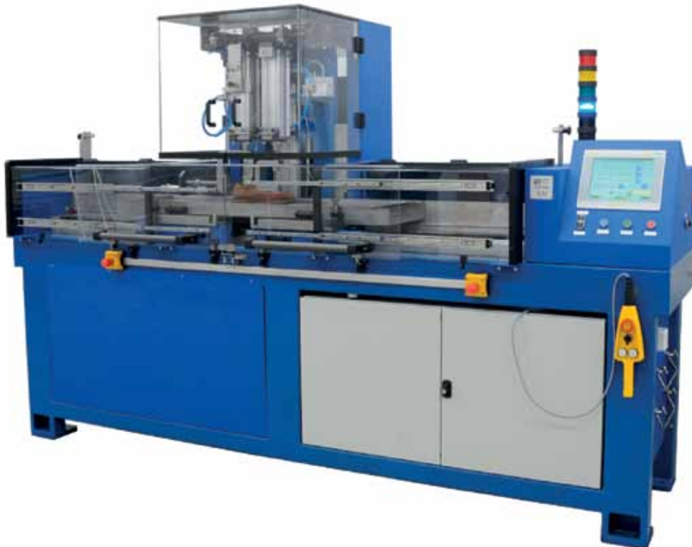
Fig. 8. Photograph of the T-31 Simulator for friction and wear testing of materials intended for shoe soles [L. 14]
