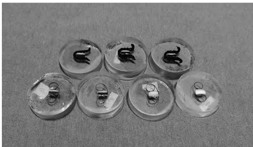
Fig. 2. Specimens for microhardness testing by the Vickers method
