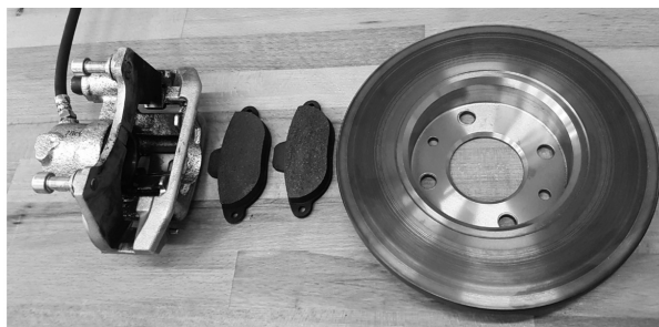
Fig. 5. The tested brake components of Cinquecento vehicle
