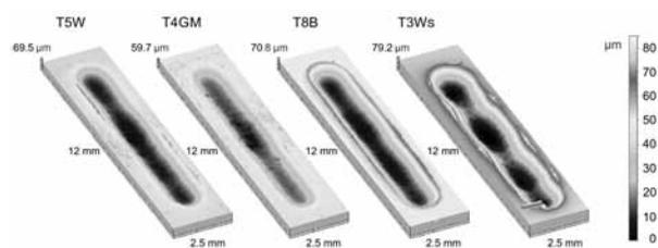
**Fig. 7. Stereometric image of friction traces**
