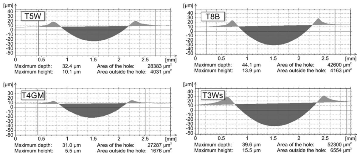
**Fig. 6. Methodology of determining the area of wear trace**
