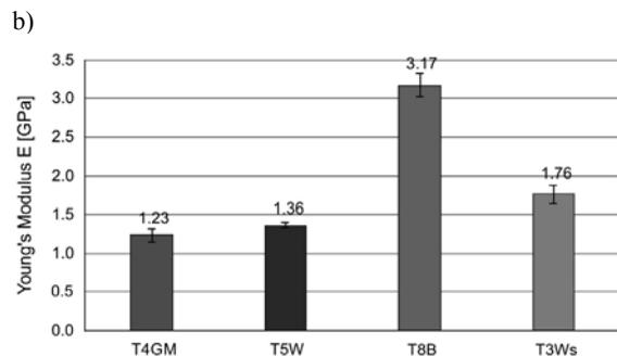
**Fig. 4. Hardness (H) and Young's modulus (E) of the tested PTFE composites**
