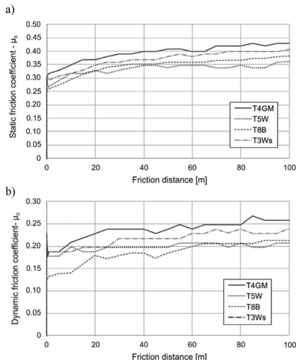
**Fig. 9. Static  $\mu_s$  (a) and dynamic  $\mu_d$  (b) friction coefficient**
