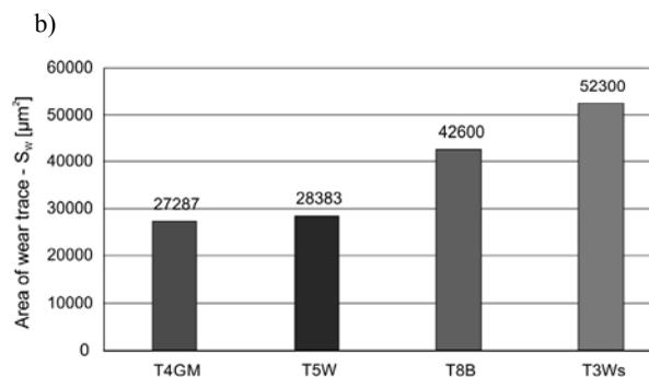
**Fig. 5. Volumetric wear –  $W_v$  (a) and area of wear trace –  $S_w$  of the PTFE composites**
