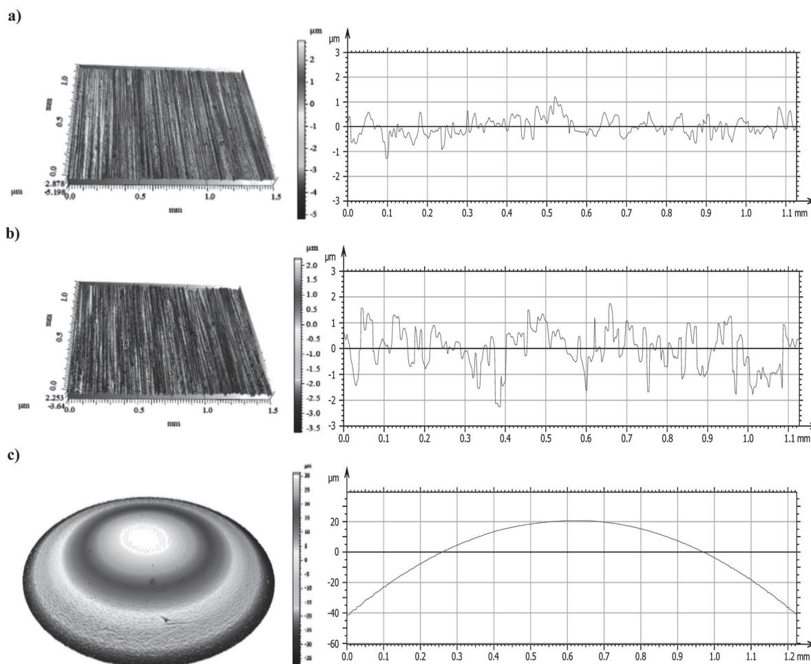
**Fig. 3.** Surface textures before the tribological tests: isometric views and primary profiles of: a) the W-DLC coated steel disc, b) uncoated steel disc, c) 100Cr6 steel ball
