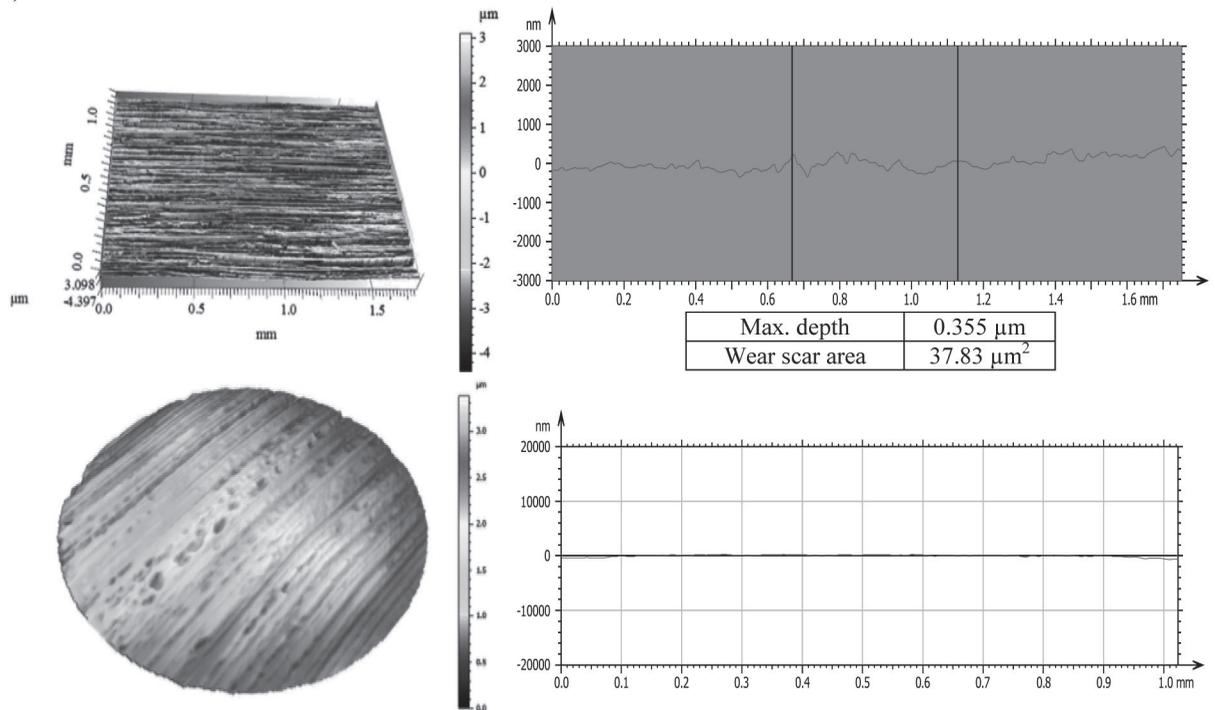
**Fig. 7. Isometric views and primary profiles of the discs and balls after the tribological tests after lubrication PAO 8 + ZDDP + C60**
