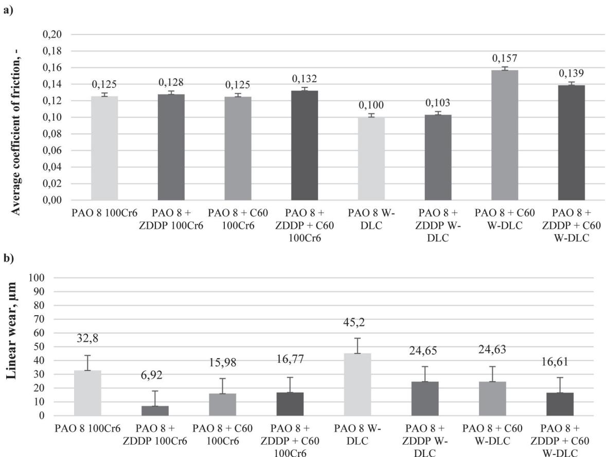
**Fig. 2. The results of the tribological tests: a) average coefficient of friction and b) linear wear**
