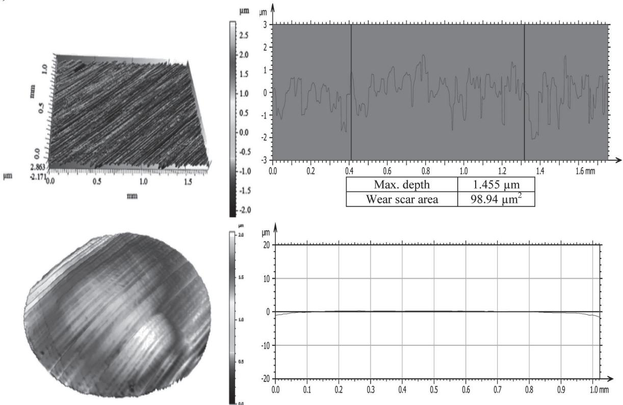
**Fig. 6. Isometric views and primary profiles of the discs and balls after the tribological tests after lubrication PAO 8 + C60**
