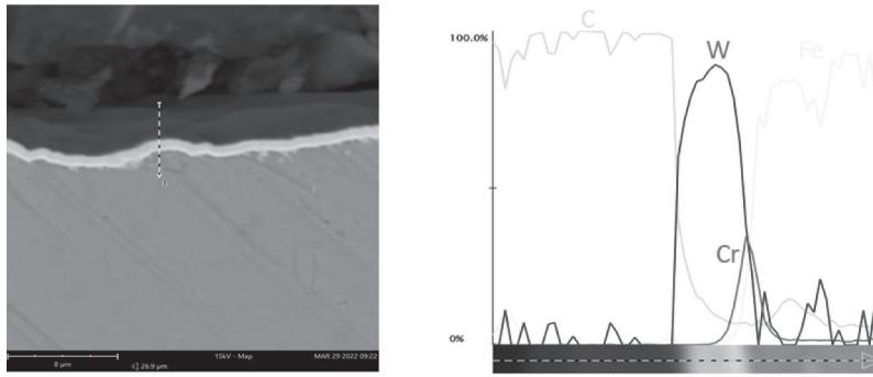
**Fig. 1. Cross-sectional view of the disc structure with EDS patterns**
