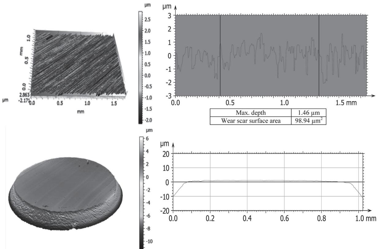
Fig. 4. Isometric views and primary profiles of the discs and balls after the tribological tests after lubrication PAO 8
