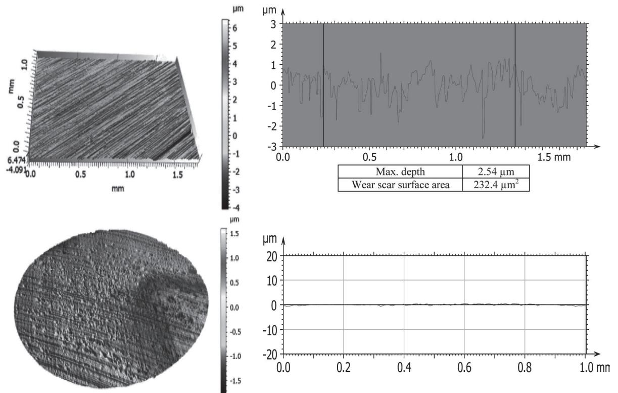
Fig. 5. Isometric views and primary profiles of the discs and balls after the tribological tests after lubrication PAO 8+ZDDP
