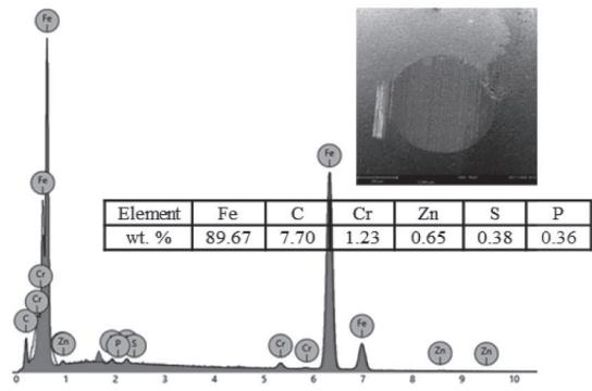
Fig. 8. EDS patterns for different points of the wear track resulting from the sliding contact of the uncoated steel discs with the steel balls
