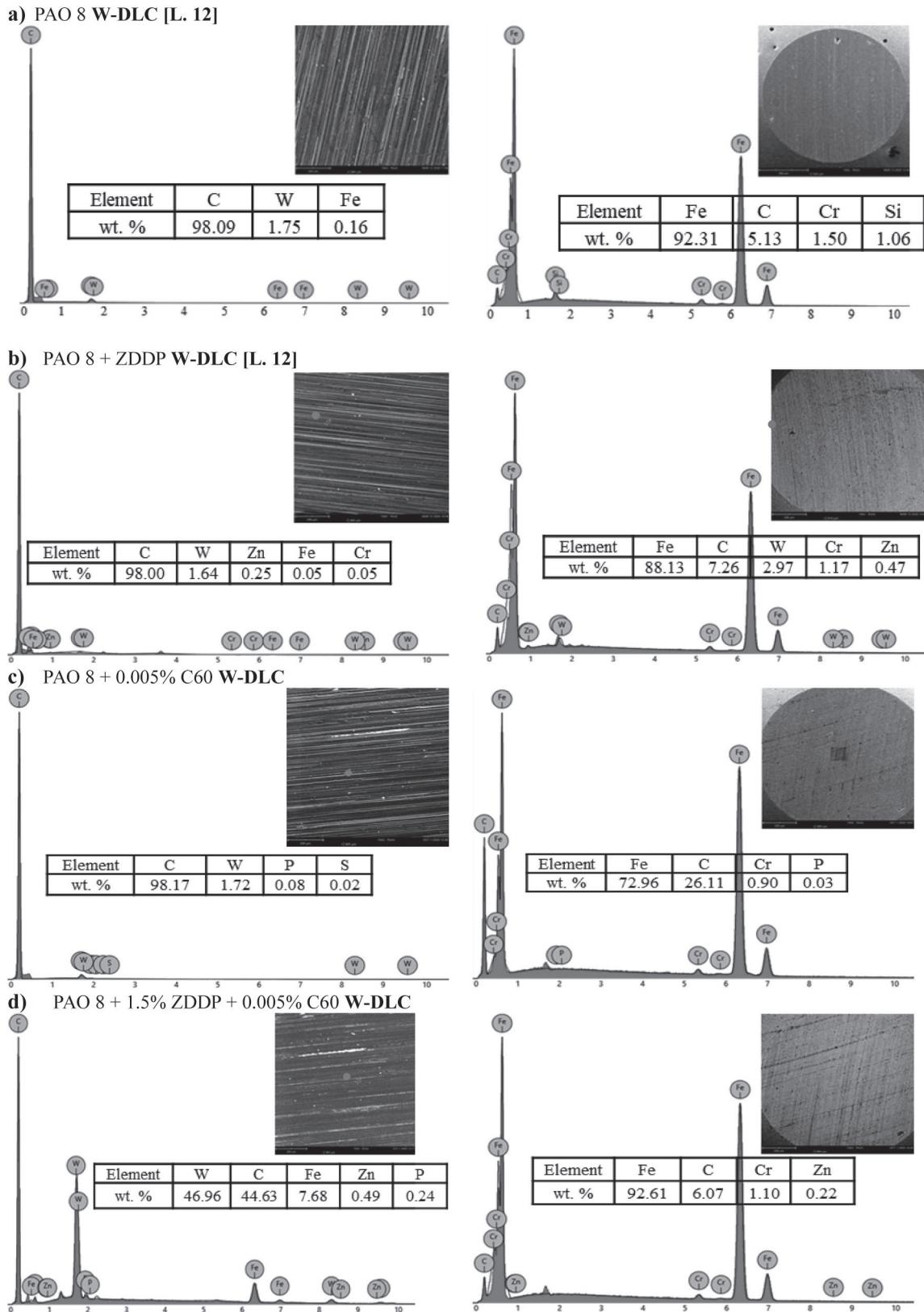
Fig. 9. EDS patterns for different points of the wear track resulting from the sliding contact of the coated steel discs with the steel balls
